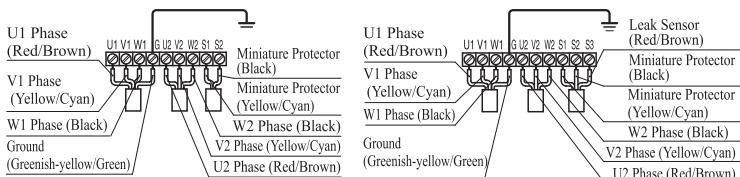
■ 3. Y-△ Starting (three cables/Non-Leak Sensor)   ■ 4: Y-△ Starting (three cables/Leak Sensor)
